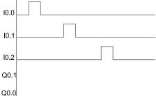
**P.3** For the given program segment i) determine the stack contents and positions after each command is executed. ii) determine the logic function Q0.0.
